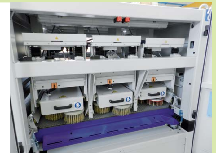
Disc Rustic machine Rusticatrice a dischi
