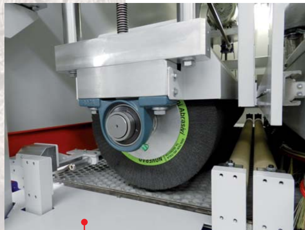
Cleaning and satining panels Pulire e satinare i pannelli
